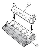
**8** Firmly press down the toner cartridge to snap into position (①).
